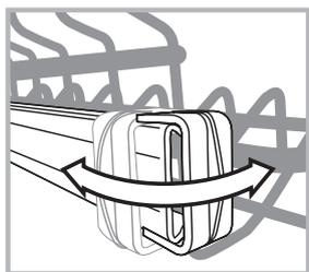
Release the two locks (right and left) and pull out the rack. When the upper rack is fitted, the locks must be always closed.
