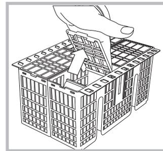
**⚠** Knives and other utensils with sharp edges must be placed in the cutlery basket with the points facing downwards or they must be positioned horizontally in the tip-up compartments on the upper rack
