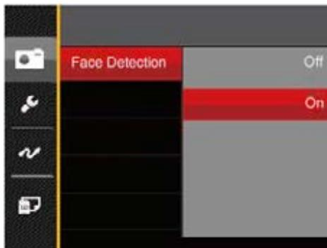
1. Hold the camera steadily and then focus on the object to detect its face. A focus frame will appear at the face on the screen when a face is detected.
