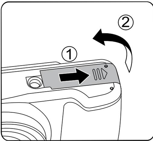
2. Insert the battery into the battery compartment according to the negative and positive directions as illustrated in the picture. Push the battery down until it locks in place.
