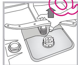
The lower sprayer arm can be removed by pulling it upwards.
