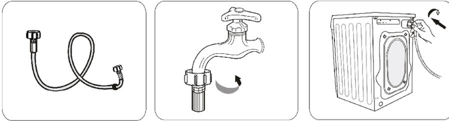
Use the new hoses supplied with the machine. Do not re-use old hoses.
