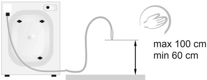
The drain hose is at the back of the machine. Fix the drain hose so that it does not move while the machine is in operation (use the elbow as shown below). Do not place the hose too deep into the outlet pipe!
