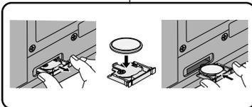
**Note:** If the holder is inserted in the wrong direction, it will not fit correctly.
