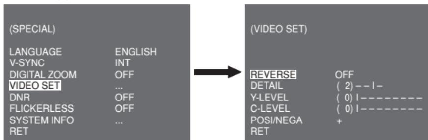
You can set the values for REVERSE, DETAIL, Y-LEVEL, C-LEVEL, and POSI/NEGA.
