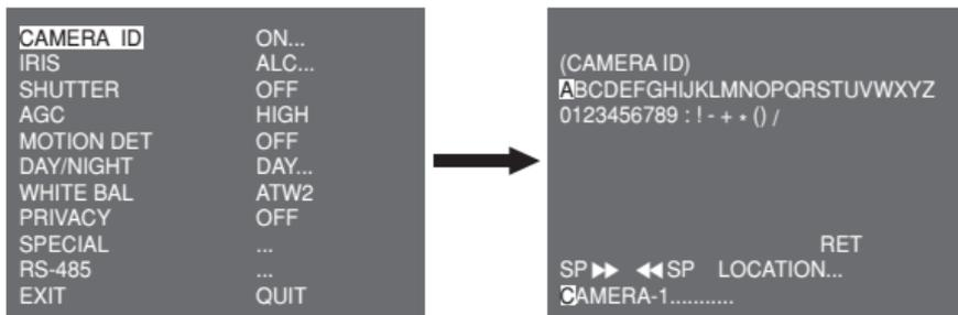
You can input a camera ID composed of alphabets, numbers, and special characters up to 20 characters long. The input camera ID can be displayed at the desired location when using the LOCATION... submenu.
