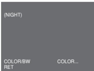
Even in night mode, you can see colour images in bright illumination. Therefore you can select any of COLOUR... and BW... In case of COLOUR..., you have to set the colour temperature for white balance. You can also specify the settings for red and blue colours on your own. In case of BW..., when the BURST is set to ON, the burst signals are output with the BW Composite Video signals. And no burst signals are output when the BURST is set to OFF.
