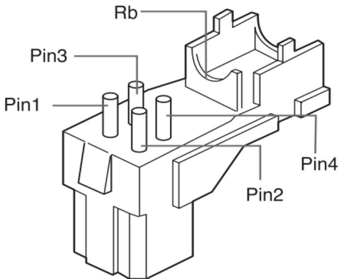
Connect each uncovered shutter control cables to the Auto Iris Lens Connector as the following:
