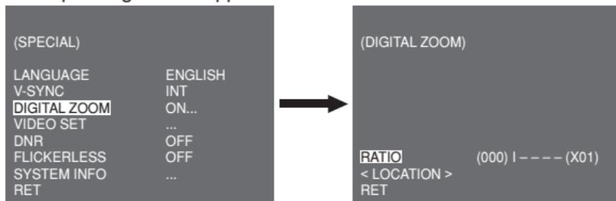
The first displayed number means the zoom ratio and the second displayed number is the magnification. When the level reaches 130, the magnification becomes 2. After the zooming position is selected, the digital zoom function applies.
