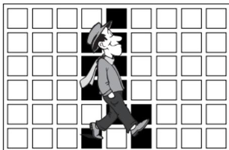
In order to set the motion detection area on your own, you have to specify the size and location for the area setting. When ON is selected in **DISPLAY**, the detected motion is displayed on the screen and the camera sends the Alarm Out signal. You can also assign the sensitivity for motion detection.
