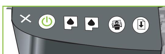
If the lights are flashing, press the power or resume button to reset the printer, and then start at the beginning of this Setup Guide.
