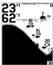
**Black** (Bottom Black) displays all pixels below the bottom contour as black, regardless of signal strength. This has the benefit of providing a high contrast between the bottom and other sonar returns on the display.
