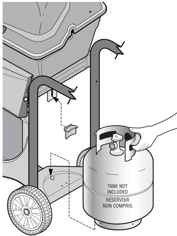
**IMPORTANT:** Ensure hose assembly does not contact the casting, or any other parts which will get hot.
