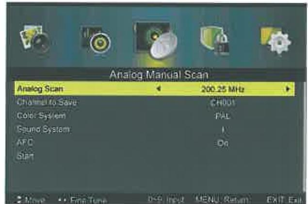
**NOTE:** Color System, Sound System and AFC will not be adjustable if there's no signal.
