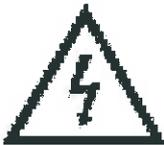
This symbol is intended to alert the user to the presence of uninsulated "dangerous voltage" within the product's enclosure that may be of sufficient magnitude to constitute a risk of electric shock of persons.
