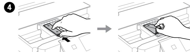
Push the tab to unlock the ink cartridge holder and then remove the cartridge diagonally.
