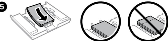
**5** Load paper toward the edge guide with printable side face-down, and check that the paper is not sticking out from the end of the cassette.
