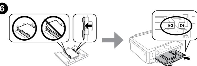
**6** Slide the edge guides to the edges of the paper. Keep the cassette flat and insert it back into the printer carefully and slowly.
