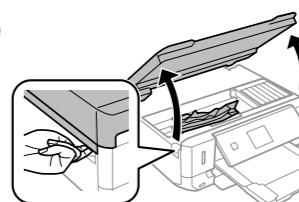
Open the scanner unit and remove all of the paper inside, including any torn pieces.
