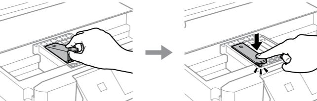
Insert the ink cartridge diagonally into the cartridge holder and gently push it down until it clicks into place.
