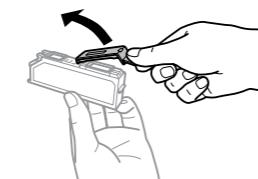
Remove the cap from the new cartridge.
