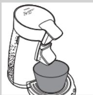
**2** Put the 1-cup pod holder □ or the 2-cup pod holder □□ in the machine without pod(s).
