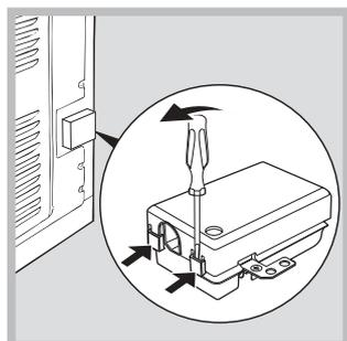
1. Open the terminal board by inserting a screwdriver into the side tabs of the cover. Use the screwdriver as a lever by pushing it down to open the cover (*see diagram*).
