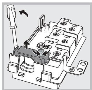
2. Loosen the cable clamp screw and remove it, using a screwdriver as a lever (see figure).
