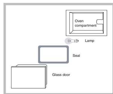
1. Remove the glass lid using a screwdriver.
