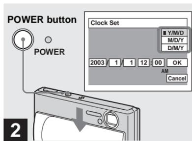
➔ Slide the lens cover or press the **POWER** button to turn on the camera.
