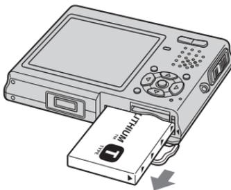
Open the battery/“Memory Stick Duo” cover, then hold the camera so that it faces downward and remove the battery pack.
