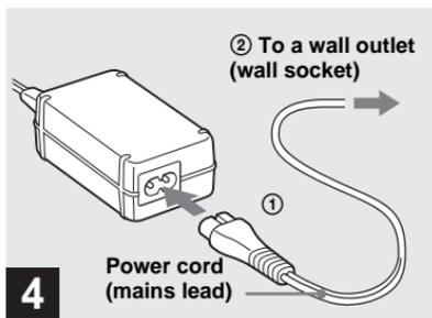
**4** → Connect the power cord (mains lead) to the AC Adaptor and to a wall outlet (wall socket).
