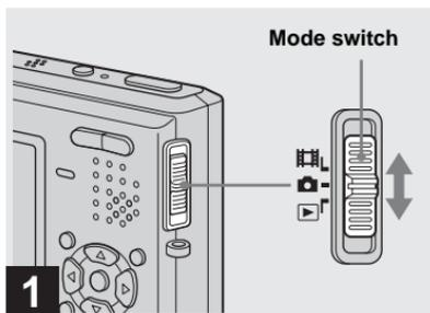
➔ Set the mode switch to
