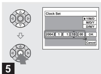
→ Set the numeric value with ▲/▼ on the control button, then press ● to enter it.
