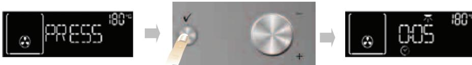
At the end of cooking time, the display shows: "PRESS TO BROWN". Press button , and the oven starts a 5-minute browning cycle. This function can be selected consecutively a maximum of twice.
