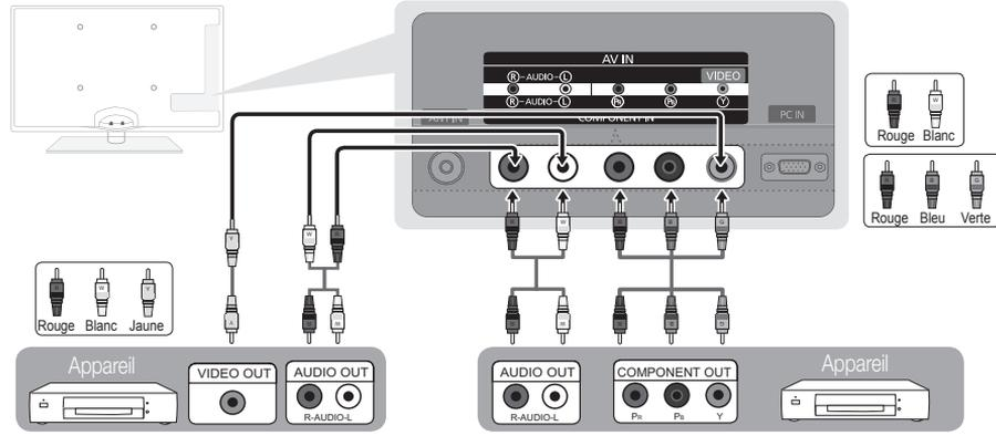
The diagram shows a television's rear panel with an AV IN section containing VIDEO, AUDIO, and COMPONENT ports, and a PC IN port. Below, two external devices are shown: the left one has VIDEO OUT and AUDIO OUT (R-AUDIO-L) ports, and the right one has AUDIO OUT (R-AUDIO-L) and COMPONENT OUT (Pr, Pb, Y) ports. Cables connect the devices to the TV ports. A legend shows red and white cables for 'Rouge Blanc' and red, blue, and green cables for 'Rouge Bleu Vert'.
