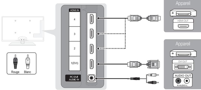
The diagram shows a television's rear panel with four HDMI IN ports (labeled 1, 2, 3, 4) and one PC/DVI AUDIO IN port. Port 1 is specifically labeled as 1(DVI). To the right, two external devices are shown: the top one has an HDMI OUT port, and the bottom one has DVI OUT and AUDIO OUT (R-AUDIO-L) ports. Cables connect the devices to the TV ports. A legend shows a red and white cable for 'Rouge Blanc' and a red and white cable for 'Rouge Blanc'.
