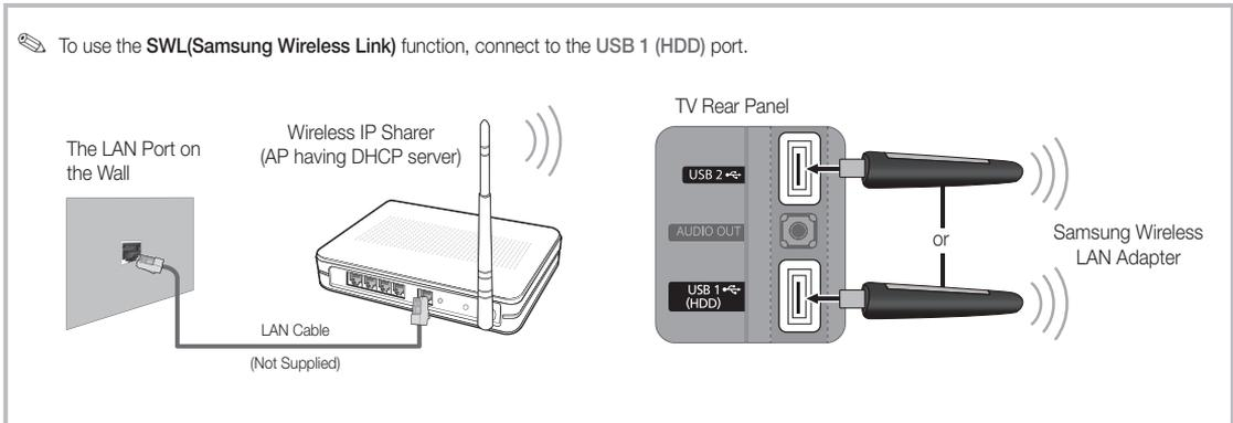
Samsung's Wireless LAN adapter is sold separately and is offered by select retailers, Ecommerce sites and Samsungparts.com. Samsung's Wireless LAN adapter supports the IEEE 802.11A/B/G and N communication protocols. Samsung recommends using IEEE 802.11N. When you play video over a IEEE 802.11B/G connection, the video may not play smoothly.
