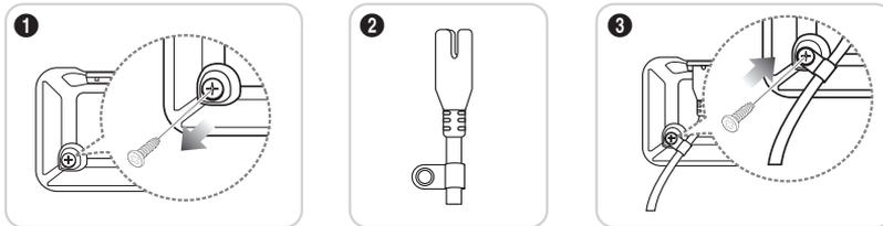
1. Remove the screw shown in the first picture above.
