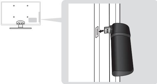
To connect the Samsung Wireless LAN Adapter using the USB right angle adapter, follow these steps:
