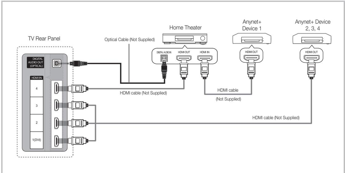
1. Connect the **HDMI IN (1(DVI), 2, 3 or 4)** jack on the TV and the **HDMI OUT** jack of the corresponding Anynet+ device using an HDMI cable.
