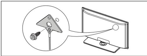
2. Firmly fasten the screw you provided (size M4xL20 or similar) to the wall or cabinet where the TV is to be installed.
