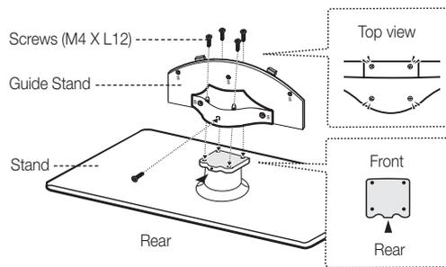
1. Connect the Guide Stand to the Stand using five screws (M4 X L12) as shown.
