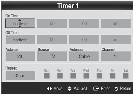
**On Time / Off Time:** Set the hour, minute, and activate / inactivate. (To activate the timer with the setting you've chosen, set to **Activate**.)
