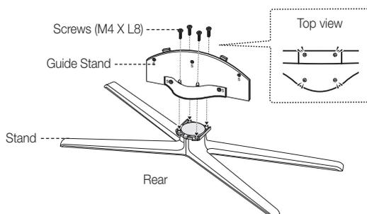
1. Connect the Guide Stand to the Stand using four screws (M4 X L8) as shown.
