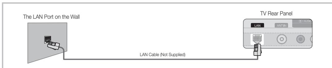
If you have a Dynamic Network, you should use an ADSL modem or router that supports Dynamic Host Configuration Protocol (DHCP). Modems and routers that support DHCP automatically provide the IP address, subnet mask, gateway, and DNS values your TV needs to access the Internet so you don't have to enter them manually. Most home networks are Dynamic Networks.
