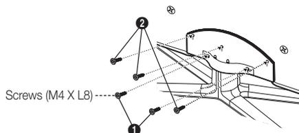
3. Fasten two screws (M4 X L8) at position ①, and then fasten three screws (M4 X L8) at position ②.
