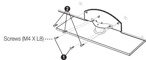
3. Fasten two screws (M4 X L8) at position ①, and then fasten three screws (M4 X L8) at position ②.
