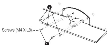
3. Fasten two screws (M4 X L8) at position ①, and then fasten three screws (M4 X L8) at position ②.
