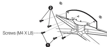
3. Fasten two screws (M4 X L8) at position **1**, and then fasten three screws (M4 X L8) at position **2**.
