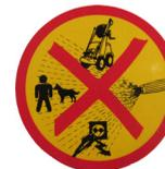
In case of improper use, the high pressure jet can be very dangerous. Do not direct jet at persons, animals or active electrical equipment or the machine itself.
