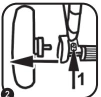
Mount the front wheels by sliding the wheel assemblies onto the prongs until they click into place.
