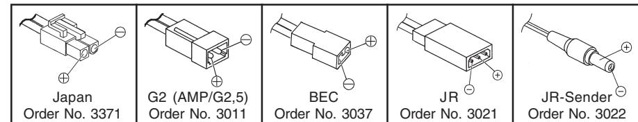
Be sure to use genuine charge leads fitted with cable of adequate conductor cross-section. All charge leads should be cut down to a maximum length of **30 cm**.
