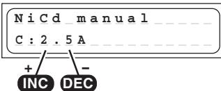
Select this program when you simply wish to recharge a battery using the set charge current. You can adjust the charge current using the INC / DEC buttons, but only **before** you connect the pack for charging. The range available is 0.1 A to 7 A. The charge process is terminated automatically in accordance with the values already set for „Ni-Cd Delta Peak cut-off voltage“.
