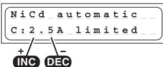
In this program the charger detects the type of Ni-Cd battery connected to it, and adjusts the charge current accordingly to avoid overcharging the pack. The maximum charge current can be set **before** you connect the battery to be charged. This is done using the INC / DEC buttons; the range available is 0.1 A to 7 A, or no restriction. The charge process is terminated automatically in accordance with the values already set for „Ni-Cd Delta Peak cut-off voltage“.
