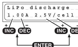
The purpose of this program is to determine the residual capacity of a Lithium pack which has not been fully discharged.
