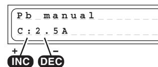
In this program you can set the maximum permissible charge current using the INC / DEC buttons, but only **before** you connect the lead-acid battery for charging. This setting only determines the top limit which the charger is permitted to feed to the battery.
