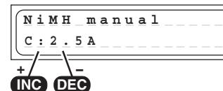
Select this program when you simply wish to recharge a battery using the set charge current. You can adjust the charge current using the INC / DEC buttons, but only **before** you connect the pack for charging. The range available is 0.1 A to 7 A. The charge process is terminated automatically in accordance with the values already set for „Ni-MH Delta Peak cut-off voltage“.
