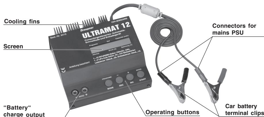
All the charger's functions are controlled by means of just four buttons. The - / DEC and + / INC buttons are used to change the current and voltage values. The function of the other two buttons varies according to the presence or otherwise of a battery at the charge sockets:
