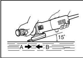
ALWAYS hold the tool firmly with one hand on housing and the other on the side handle. Turn the tool on and then apply the wheel or disc to the workpiece.
