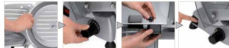
Attach the blade shield to the back plate. Den Schleifschutz anbringen.
