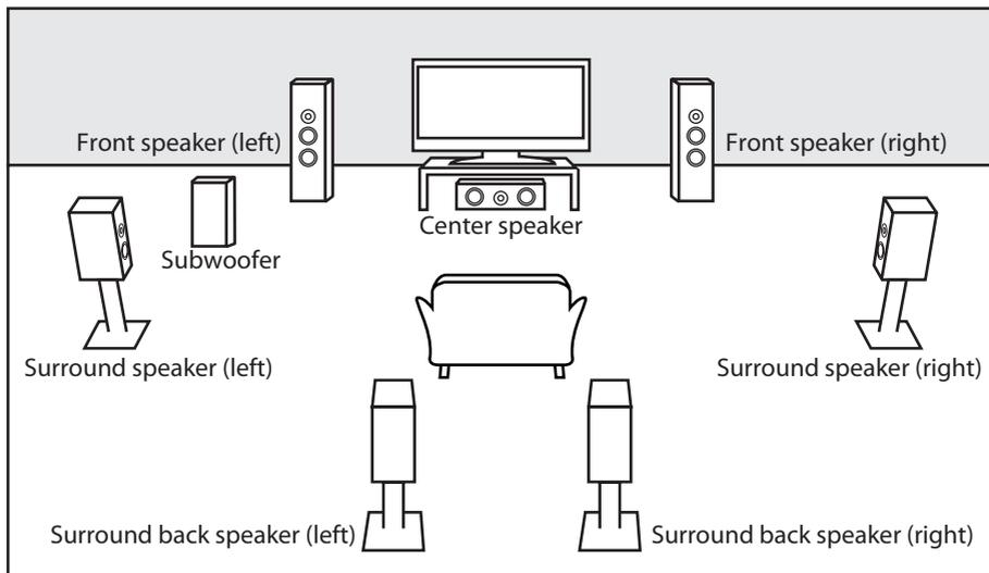
To make the most of its feature, set up your speakers appropriately by referring to the table below. Speaker setting options are available in Setup → Quick → HDMI Audio Out → HDMI Multi(LPCM) or Setup → Custom → Audio → HDMI Audio Out → HDMI Multi(LPCM).
