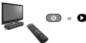
4. When the device responds correctly, press **OK**. Three long flashes indicate that the operation has been carried out **correctly**.
