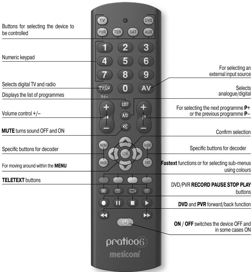
**Before using the remote control, insert the batteries and programme it.**
