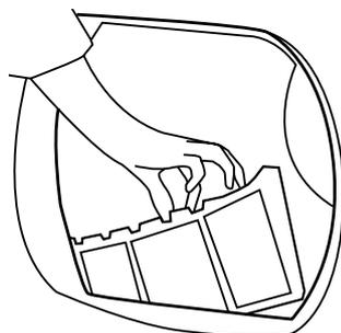
**IMPORTANT:** To maintain the efficiency of the dryer check that the fluff filter is clean before each drying cycle.
