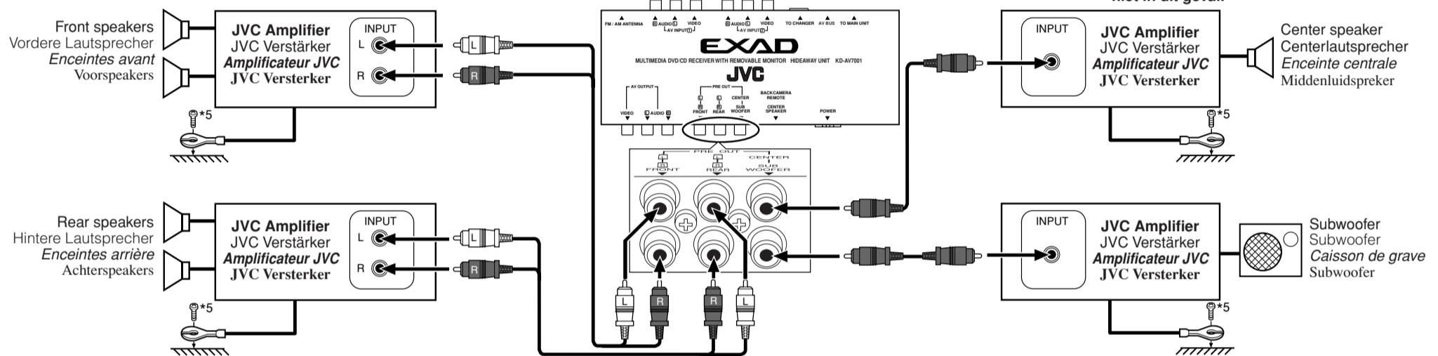
\*<sup>5</sup> Firmly attach the ground wire to the metallic body or to the chassis of the car—to the place uncoated with paint (if coated with paint, remove the paint before attaching the wire). Failure to do so may cause damage to the unit.
