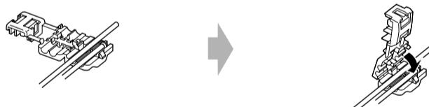
Contact the metallic part of the crimp to the wires inside.
