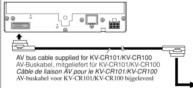
AV bus cable supplied for KV-CR101/KV-CR100
