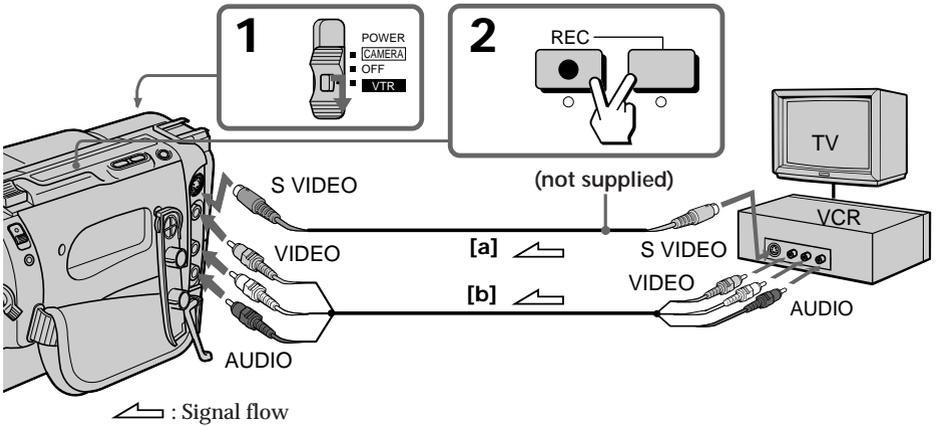
If your VCR or TV has an S video jack, connect using the S video cable (not supplied) [a] to obtain a high quality picture.
