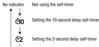
Press the shutter button, the self-timer lamp flashes, and a beep sounds until the shutter operates.
