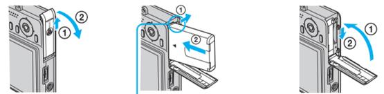
Open the battery/"Memory Stick Duo" cover. Insert the battery pack while pressing the battery eject lever with the tip of the battery. Close the battery/"Memory Stick Duo" cover.
