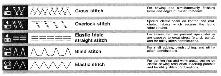
Then turn the outer ring of the stitch selector until the number indicating the desired stitch length (between 0 and 2) is opposite the mark. Now your machine is ready for sewing an elastic seam.
