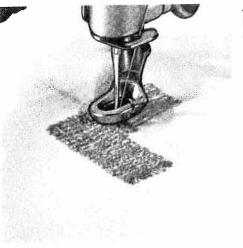
After you have finished darning, swing the reverse-feed control back to its regular sewing position.
