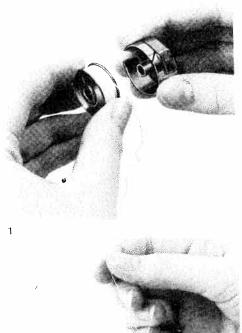
Fig. 1: Insert the filled bobbin into the bobbin case, making sure the thread end drops from the top down towards you.
