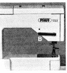
2. **Position B** (illustrated above) is used when you need to turn the fabric. The sewing foot is raised, but the needle remains in the fabric and serves as a pivot point for turning the material.
