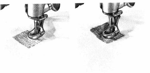
Hold the material flat with both hands. Stitch back and forth across the hole lengthwise, with the machine running at high speed. Be sure the stitches are closely spaced. Then turn the fabric at right angles and sew back and forth over the preceding work with short stitches. This anchors the threads in the unworn area around the hole.
