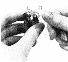
The **lower tension** is regulated by turning the small knurled screw on the bobbin case. Turn this screw to the right (with your thumb rather than your finger nail) for a tighter tension, or to the left for a looser tension. Right (R) and left (L) are indicated by arrows.
