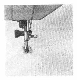
To make different size cording, the following twin needles and cording feet can be obtained from any Pfaff dealer:
