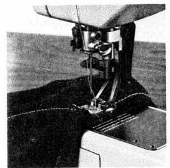
Even the thickest cross seams are no obstacle for the electronic Control of the Pfaff 1222-E.
