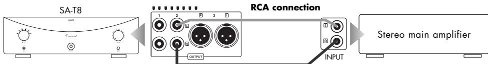
You can as well use all three stereo outputs at the same time, giving way for up to 6 main amplifier channels to supply their loudspeaker. For that all you need to do is connect all remaining stereo outputs (8) with additional main amplifier channel inputs.
