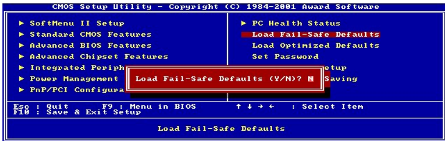
Figure 3-12. Ecran du Load Fail-Safe Defaults
