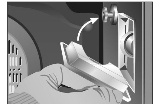
The replacement bulb must be resistant to temperatures up to 300 °C. You can order one from Technical Service.
