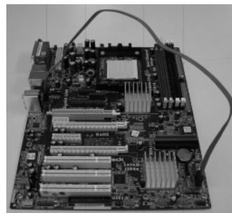
Connect the SATA data cable to the red eSATAII connector (eSATAII_BOTTOM)
