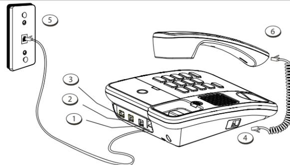
1. Adjust the **RINGER** volume switch to the desired setting. Default setting is **HI**.
