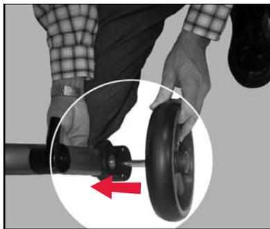
Slide the rear wheel axle into the housing on the side of the rear wheel assembly. Pull wheel to ensure that it is secure.
