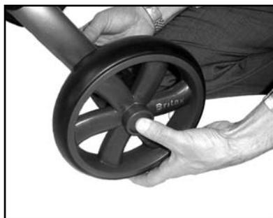
2 Press the release button at the center of the wheel and pull wheel from wheel assembly.
