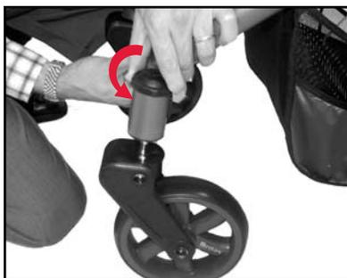
1 Raise front of stroller and twist the release knob on the top of each front wheel assembly (as indicated by arrows).
