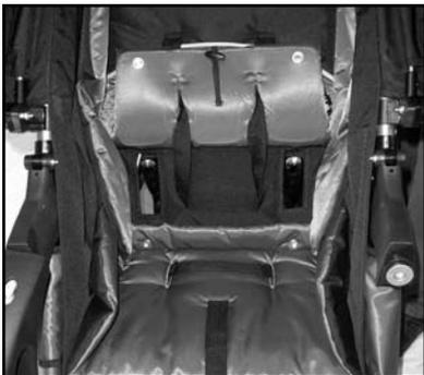
4 Secure flap with toggle and loop, making sure that the harness is stored behind flap when it is secured.
