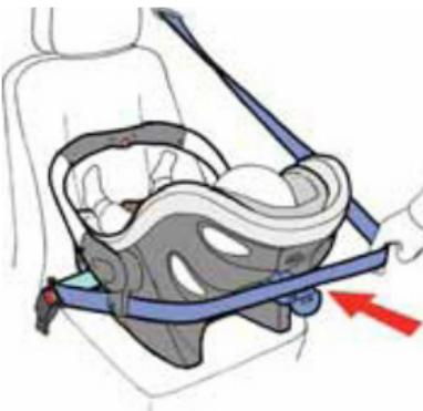
Tighten that part of the strap and shut the locking clip (02). Make sure that the seat is firmly fastened by pulling on it.
