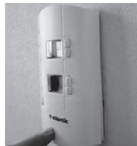
7/ After programming the card (see Page 17), refit the cover or the cover and programming card assembly, depending on the model.
