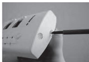
3/ Insert a flat screwdriver in the spur next to the screw and lift to open the wall box. Separate the front section from the base section.
