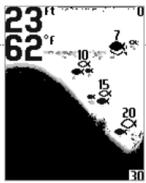
**Black (Bottom Black)** displays all pixels below the bottom contour as black, regardless of signal strength. This has the benefit of providing a high contrast between the bottom and other sonar returns on the display.
