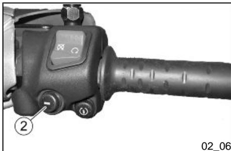
When the total odometer function is seen on the multifunction display «1» hold the MODE button «2» down for more than three seconds. The colon between the hours/minutes will begin to flash.
