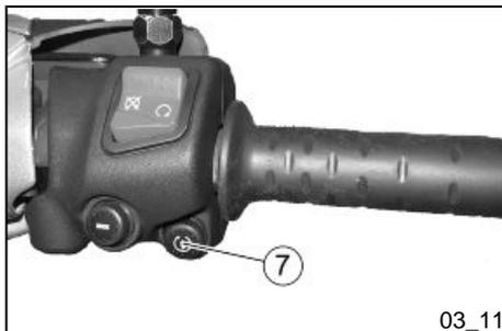
Press the start up button «7» and allow the starter motor to work for about five seconds without accelerating.
