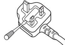
**How to replace the fuse:** Open the fuse compartment with a screwdriver and replace the fuse.
