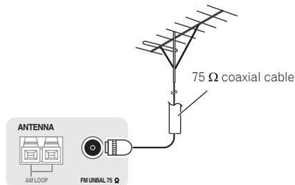
To improve AM reception, connect a 5 m to 6 m length of vinyl-coated wire to the **AM LOOP** terminals without disconnecting the supplied AM loop antenna.
