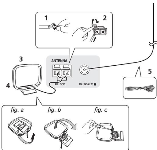
**1 Pull off the protective shields of both AM antenna wires.**
