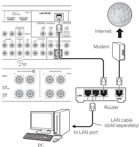
Connect the LAN terminal on this receiver to the LAN terminal on your router (with or without the built-in DHCP server function) with a straight LAN cable (CAT 5 or higher).
