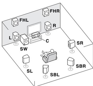
A 9.1 ch surround system connects the left and right front speakers (**L/R**), the center speaker (**C**), the left and right front height speakers (**FHL/FHR**), the left and right surround speakers (**SL/SR**), the left and right surround back speakers (**SBL/SBR**), and the subwoofer (**SW**).
