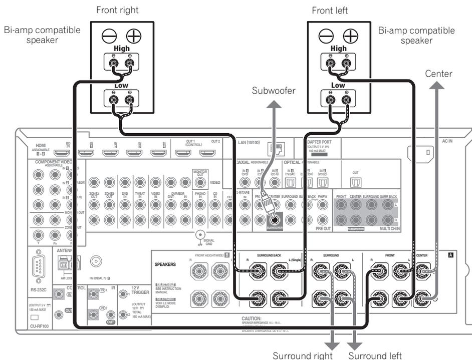
Bi-amping is when you connect the high frequency driver and low frequency driver of your speakers to different amplifiers for better crossover performance. Your speakers must be bi-ampable to do this (having separate terminals for high and low) and the sound improvement will depend on the kind of speakers you're using.
