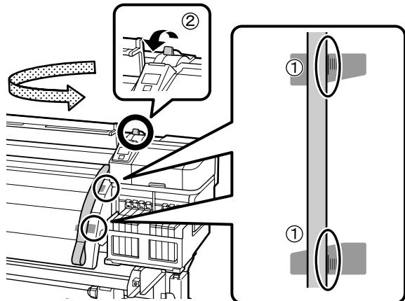
From the front of the printer, align the right edge with the longest marks on the scales at the center of the labels.
