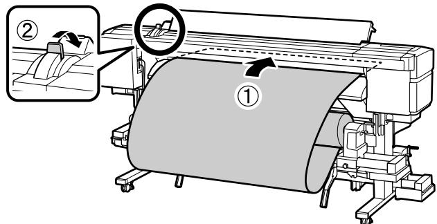
If the left end of the media is not at the center of the rectangular area as shown in the figure on the right, return to step [4].
