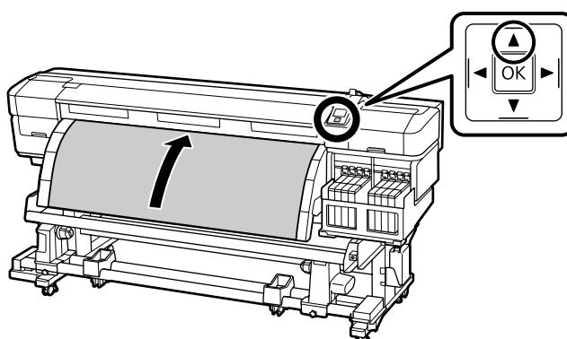
If the media is loaded printable side in, press the ▼ button to rewind the media. We recommend that you press the ► button in the control panel and set **Media Suction** to 2.
