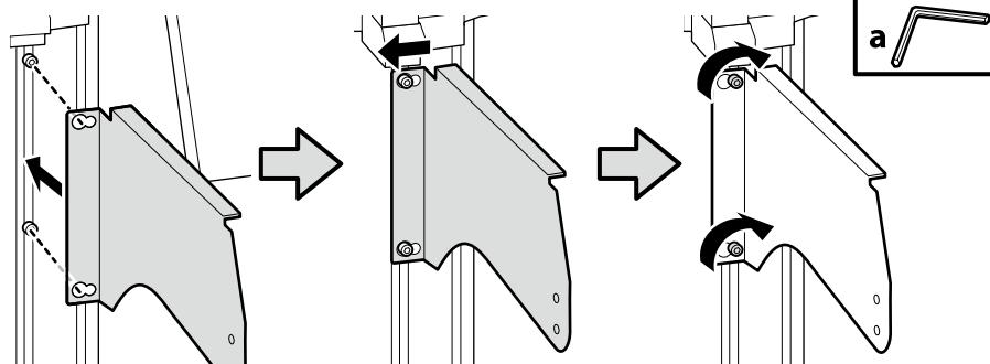
Fully tighten the two screws that you provisionally tightened.
