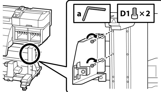
Temporarily fasten the two screws as shown in the figure.
