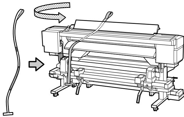
Position the rolled side of the film at the top, and insert it into the printer.
