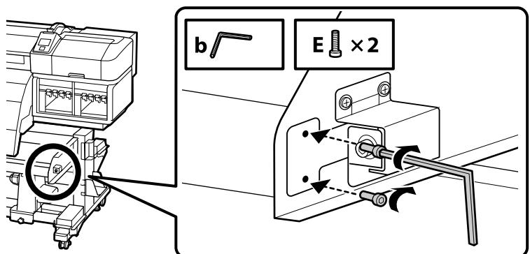
Keep the two screws shown in the figure temporarily tightened until the parallel adjustment is completed.
