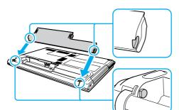
Unlock the battery's **LOCK** switch before installing the battery, and then lock the switch after installing.
